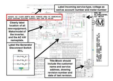
Figure 2 - Required Elements of an Acceptable Drawing
