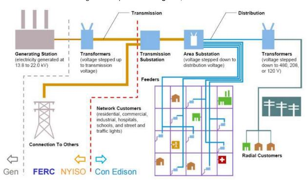
Figure 1 - Electric Distribution System
