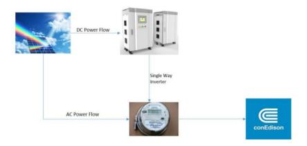
Figure 5 - Exclusive ESS Charge from PV Configuration
