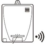
Transmits an end-of-service-life notification during the health checks performed every 8 hours.
