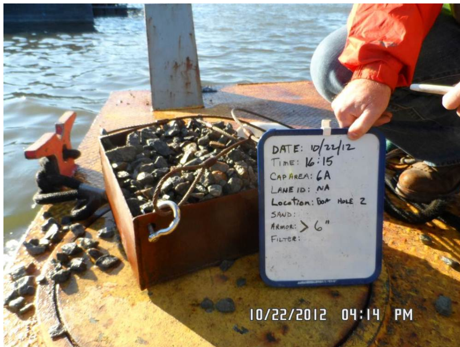
Photo 3: Armor thickness verification in Cap Area 6A.
