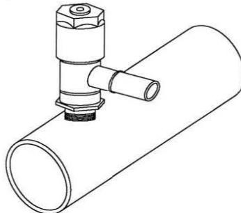
FOR CAST IRON MAINS (8" AND LARGER), DRILL AND TAP THE MAIN AND CONNECT THE BRASS-BASED TEE DIRECTLY TO THE MAIN WITHOUT A STRAP SADDLE. NO ANODE IS NECESSARY.
