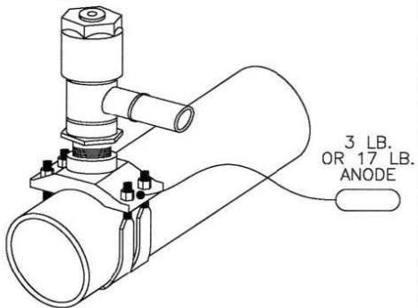
FOR PROTECTED STEEL, CAST IRON (6" AND SMALLER) OR WROUGHT IRON MAINS, DRILL THE MAIN ONLY AND CONNECT THE BRASS-BASED TEE USING AN INSULATED STRAP SADDLE. ATTACH A 3 LB. MAGNESIUM ANODE TO 6" AND SMALLER STRAP SADDLES AND A 17 LB. MAGNESIUM ANODE TO 8" AND LARGER STRAP SADDLES.
