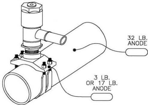
FOR UNPROTECTED STEEL MAINS, DRILL THE MAIN ONLY AND CONNECT THE BRASS-BASED TEE USING AN INSULATED STRAP SADDLE. ATTACH A 3 LB. MAGNESIUM ANODE TO 6" AND SMALLER STRAP SADDLES AND A 17 LB. MAGNESIUM ANODE TO 8" AND LARGER STRAP SADDLES. INSTALL A 32 LB. "HOT SPOT" MAGNESIUM ANODE TO THE PIPE.
